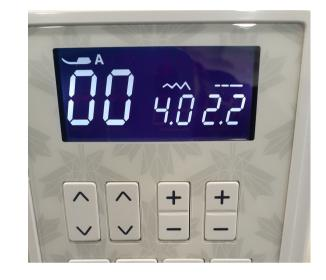
With the machine still set on straight stitch, move the needle position to the right by pressing the plus sign until it gets to 4 (you can see the little zig-zag icon above the number 4) and press the minus sign under the stitch length icon (just above the number 2.2) to make the stitch length shorter.
